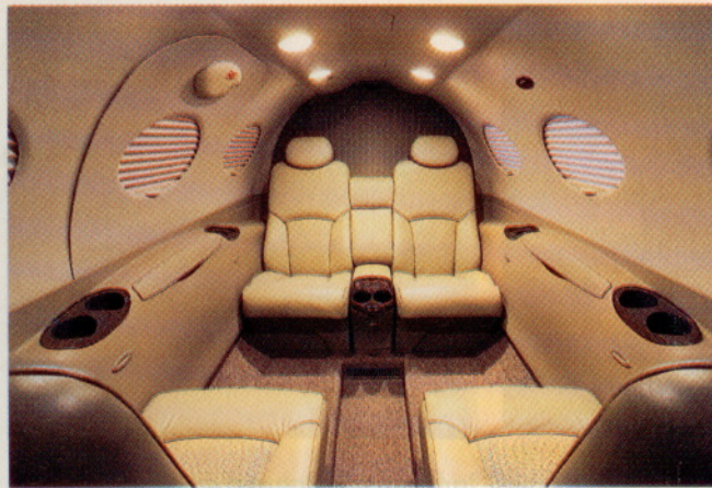
Six elliptical windows at passenger eye level give the cabin a roomy feel; pleated shades can be raised up to keep the sun out. The cabin fuselage area is a constant 55 inches wide. A four-inch dropped aisle extends for the length of the cabin.
